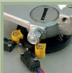
Prepared for the installation of electromechanical water-proof limit switches
