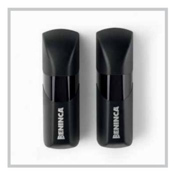
**PUPILLA.F** Pair of fixed photocells for external fitting. Compact dimensions 110 x 36 mm, height 31 mm. 24 Vdc power supply. A led makes the centring of the beam easy and fast
